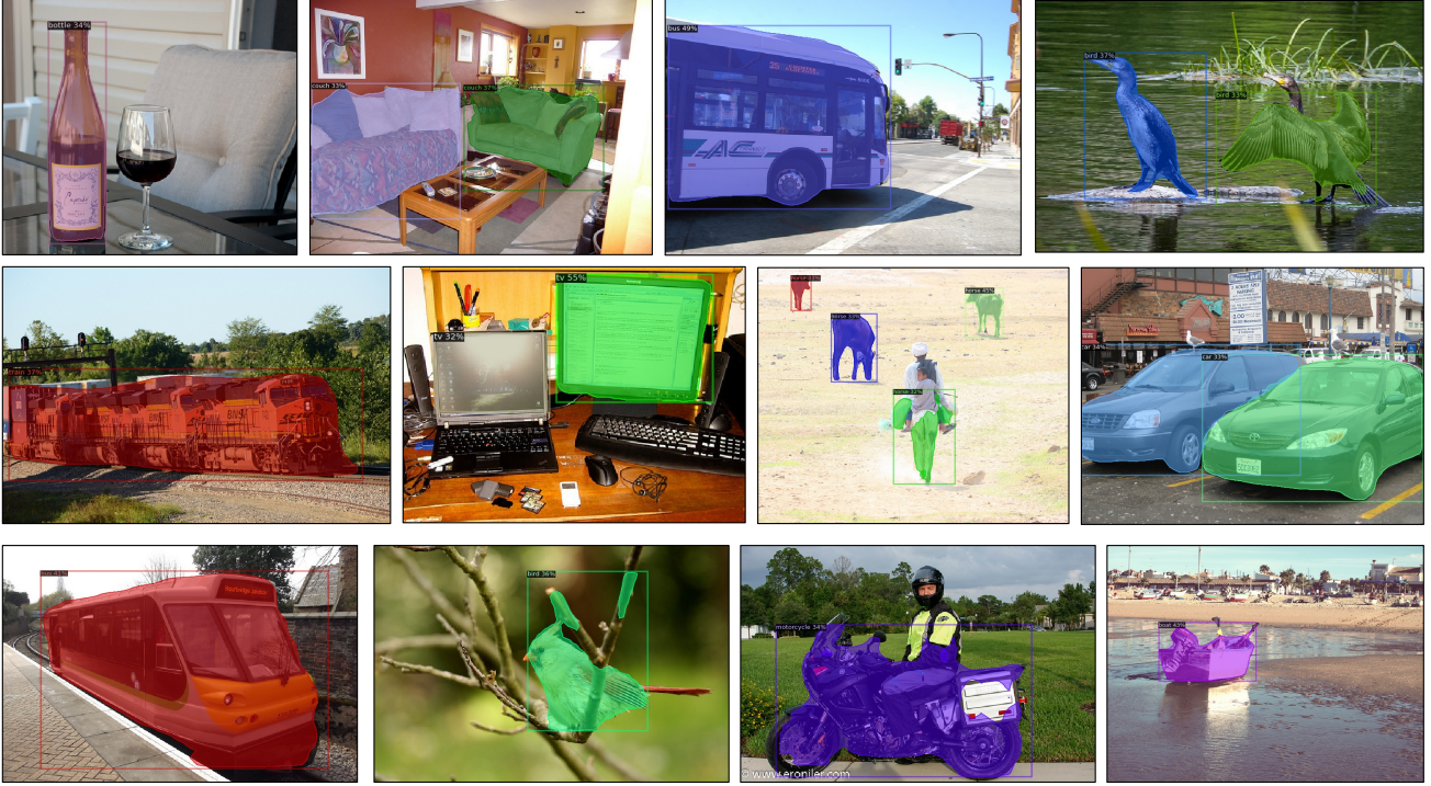
Figure 3. Representative results of iFS-RCNN on COCO-new with K = 30 . The top two rows show success cases while the bottom row shows failure cases. In the last row, from left to right: the train is detected as bus, bounding-box is too large for the bird, the human leg is segmented as a part of the motorbike, the small boats far behind are not detected.
