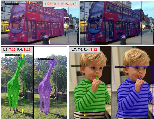
Figure 4. Bounding-box refinement with our uncertainty-guided box predictor on COCO-new with K = 1 . For each pair, left: initial box, right: refined box. The box labels show left (L), top (T), right (R), and bottom (B) side uncertainties; red text indicates high uncertainty ( \geq 10 ) that lead to large refinements. Yellow arrows indicate the refined direction of each box side.
